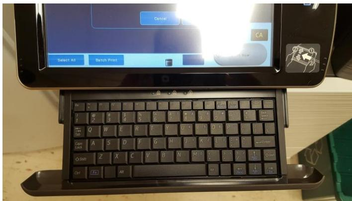
Input the code using the pull out keyboard. Grab from the bottom of the control panel and extend towards yourself.
